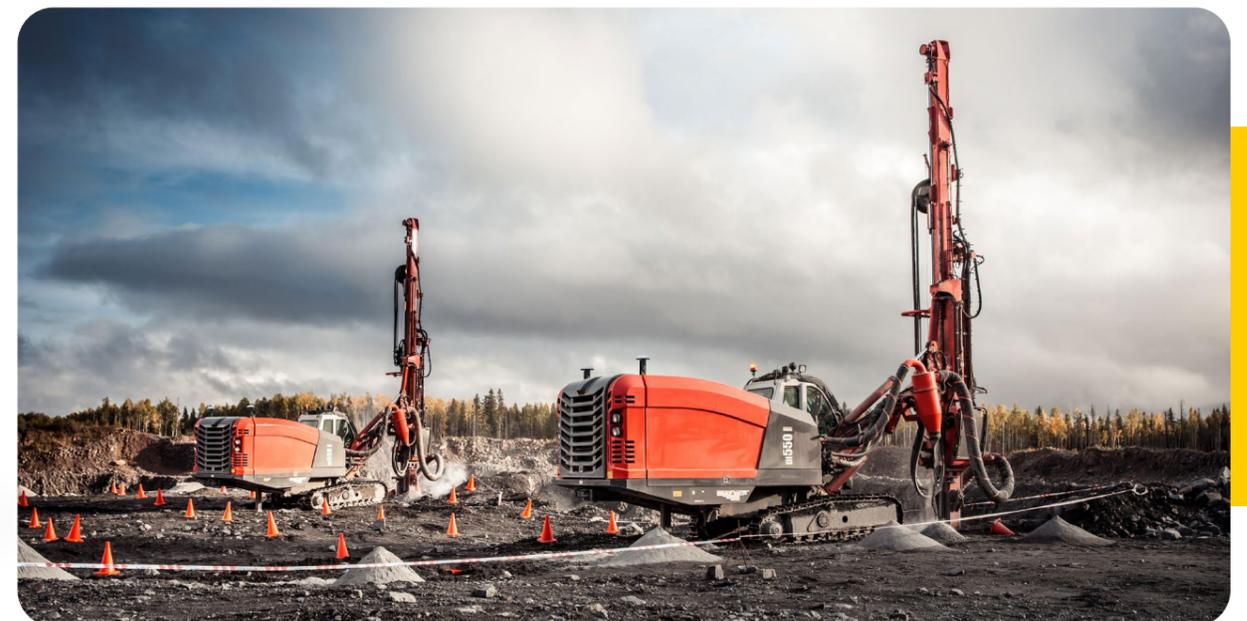
Documenting as-built with Xsite® PRO 3D is made easy for the operator. After a hole is finished, the system stores the hole's as-built data automatically.
