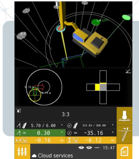
Finished holes are easy to separate from the system's screen from the green color.
